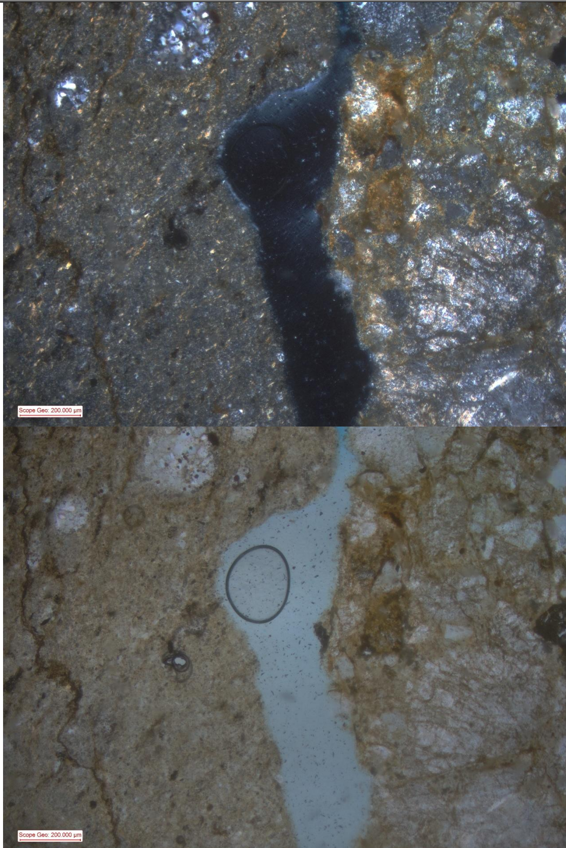
Micrograph taken in cross (top) and plane (bottom) polarized light, at low magnification. The image shows two fragments on the left are a very fine mudstone with rare very fine clasts of quartz and radiolarian infilled with microcrystalline quartz within a clay cemented matrix. The fragment on the right is more coarse grain sandstone that has been largely altered to clay forming a muddy sandstone.
